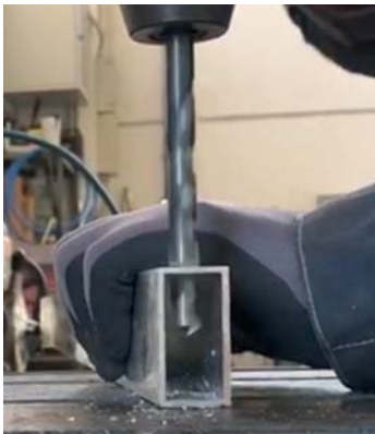
1. Create the hole on the aluminum profile as per drawings specs.
