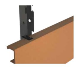
4. NOTE: the clip has to slot in the substructure.
